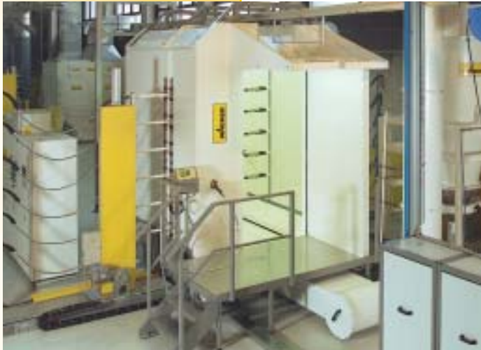
Fixed integral booth floor with blow-out device
